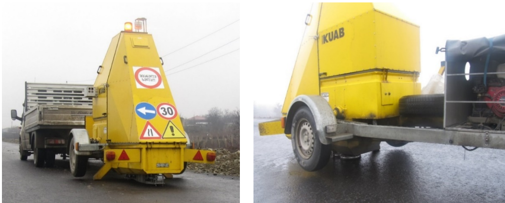
Fig. 1. Falling Weight Deflectometer FWD KUAB 50 during testing
